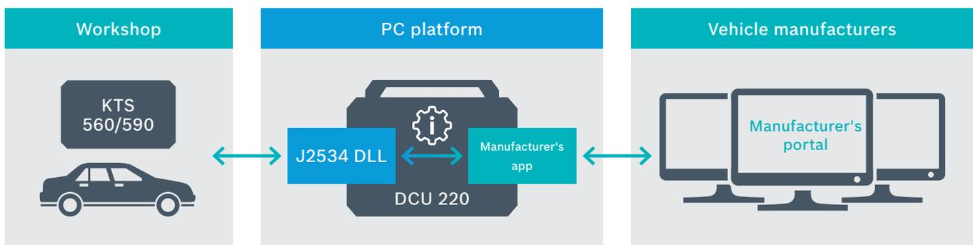
KTS 560/590 can today be used with Euro 5/6 PassThru for the following vehicle manufacturers: Audi, BMW, Citroën, Ford, Land Rover, Mercedes-Benz, Opel, Peugeot, Renault, Seat, Škoda, Toyota, Volkswagen and Volvo.
